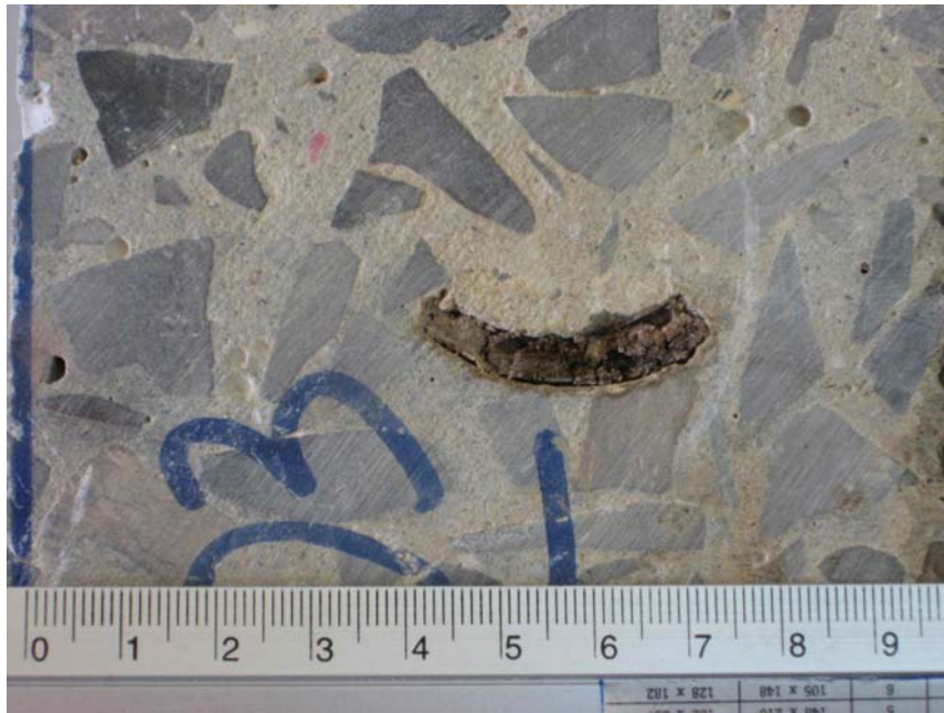
Figure 5.2 The condition of the bamboo after six years within a cut block (No 3)
