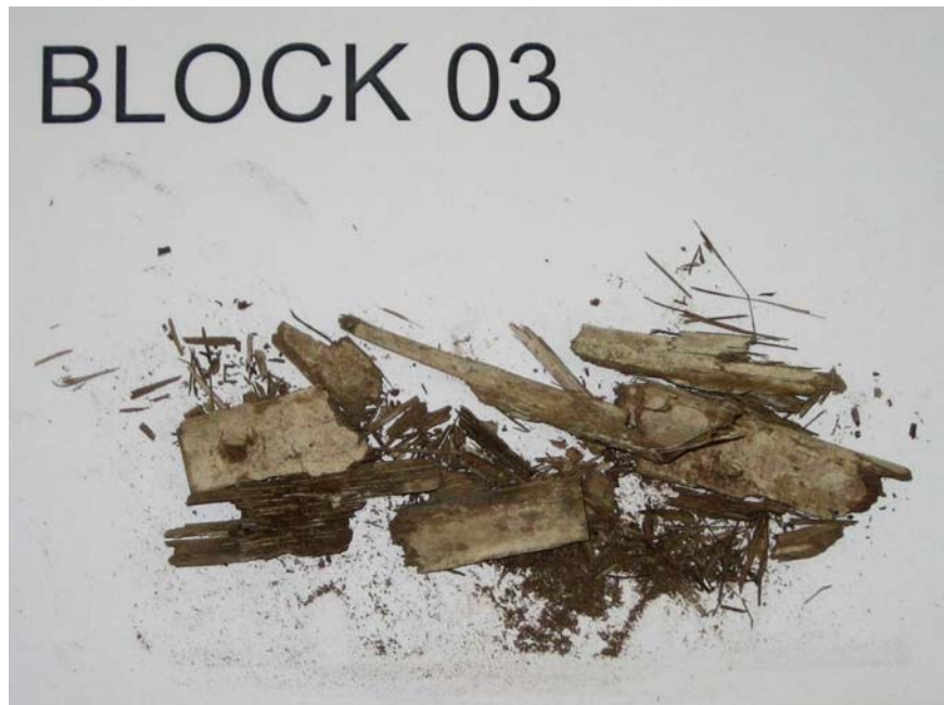
Figure 5.3 The condition of the bamboo after extraction from crushed block (No 3)
