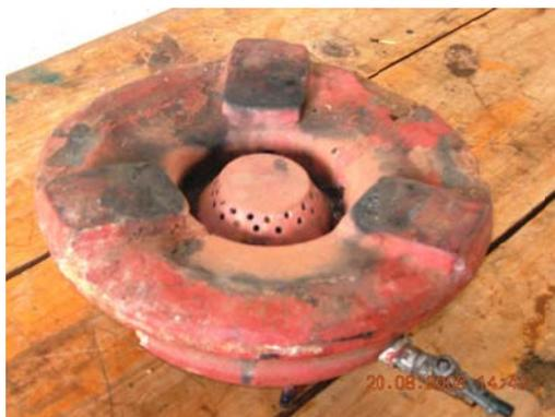
A biogas burner developed in Tanzania
