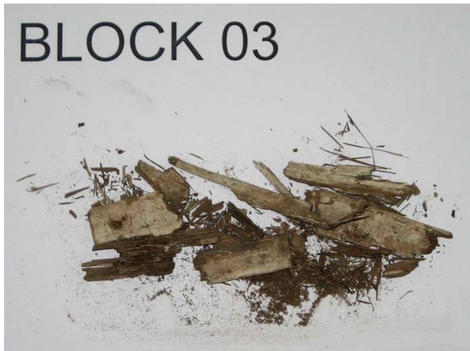
The condition of the bamboo after six years within a cut block (No 3)
