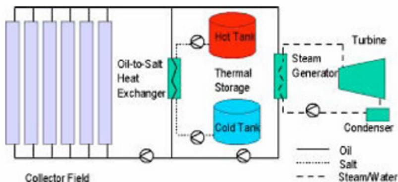
Figure 12: Two-Tank Indirect Storage System (Source: NREL)
