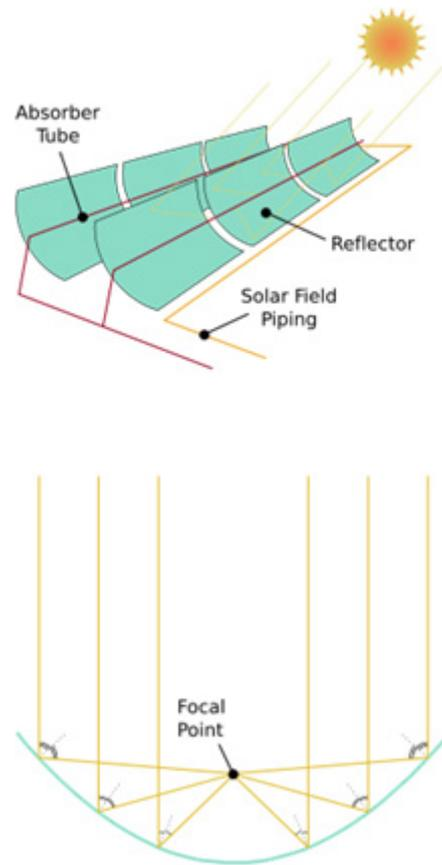
**Figure 3: Principles of solar parabolic trough collector (Source: Andrew Buck)**
