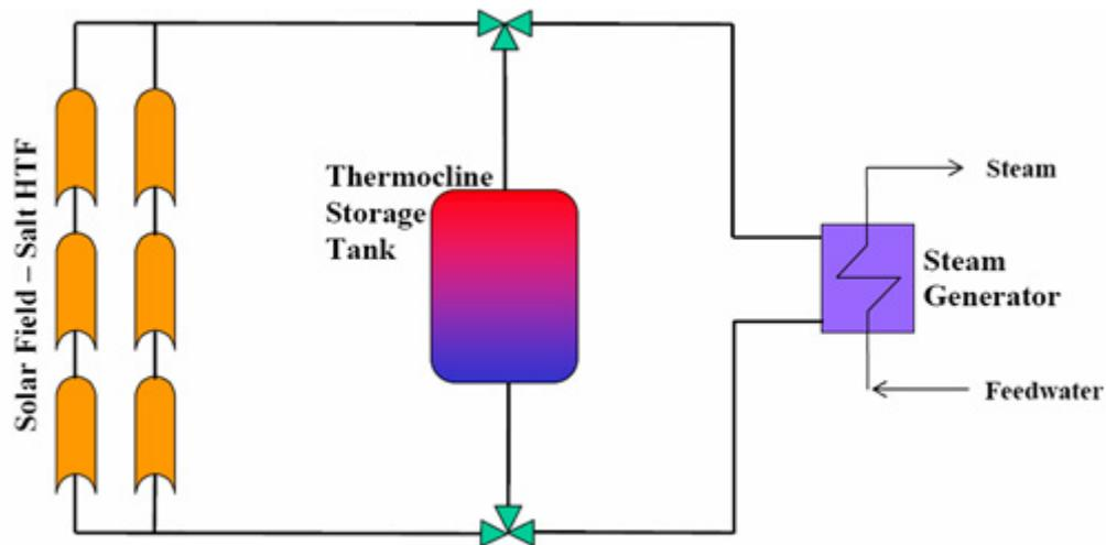
Figure 14: Single-Tank Thermocline Storage System with Direct Molten Salt (Source: NREL)
