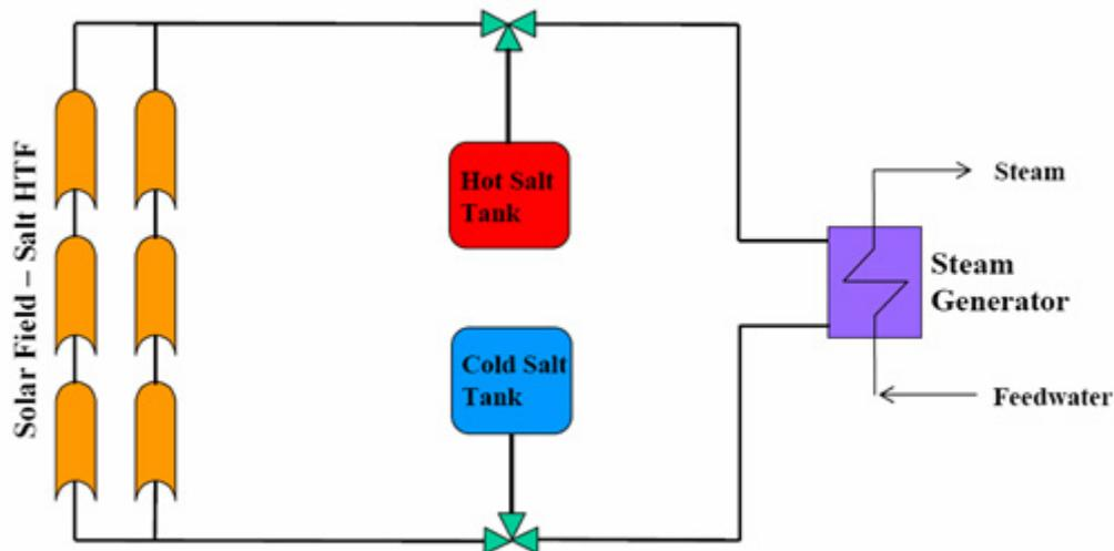
**Figure 13: Two-Tank Direct Molten Salt Storage System (Source: NREL)**
