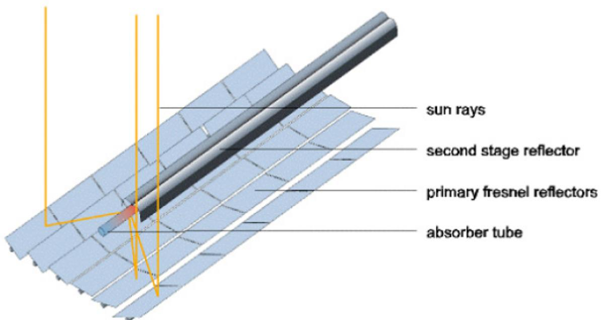
Figure 6: Principle of a linear Fresnel solar collector
