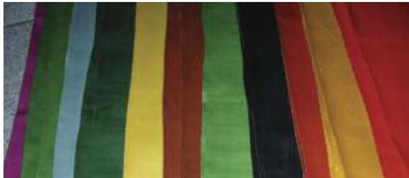
Colourful lamina of rubber-impregnated cloth for making bags (R Putz) and local production of lamina using traditional vulcanisation methods
