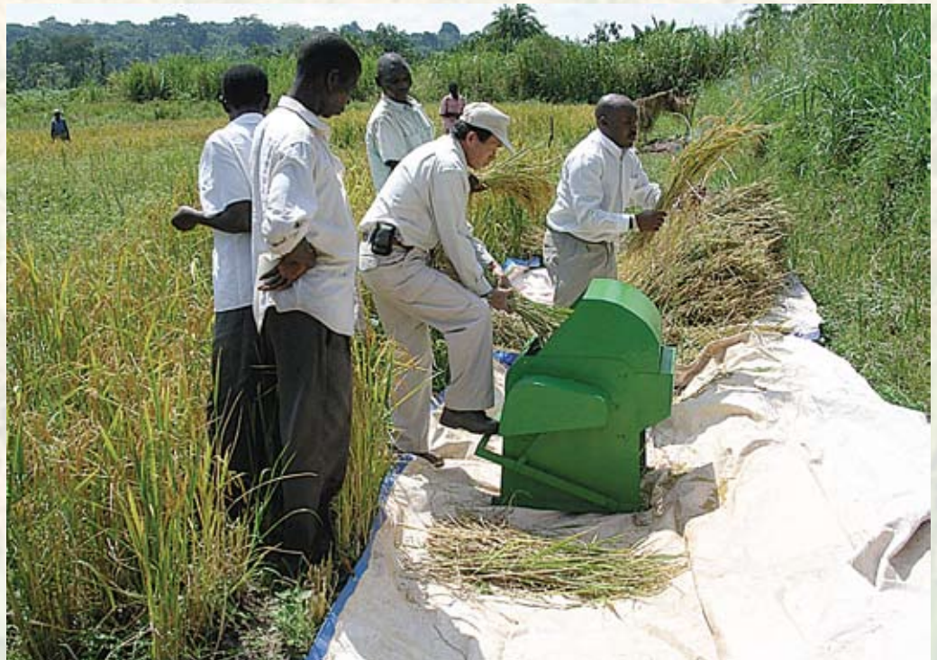
Mr. Tsuboi from JICA - Namulonge demonstrates how to use a pedal thresher
