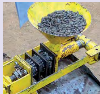
Figure 7.31 – Extracting oil from jatropha seeds using a press
