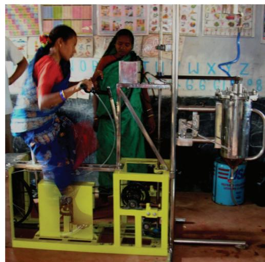
Figure 6: Pedal-driven biodiesel reactor (Photo: CTxGreEn)
