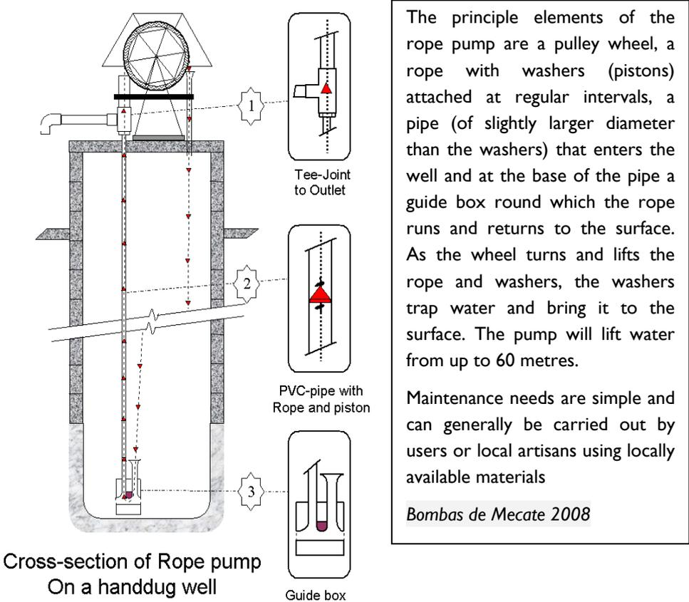
The basic design (see Figure I-1) has been provided with varying degrees of protection some of which have added significantly to the cost. Accompanying data on water quality changes are lacking, however, and encasing the top works (one option) hides the state of the rope and may encourage greater corrosion. The basic rope pump is usually installed to conform to JMP definitions of
