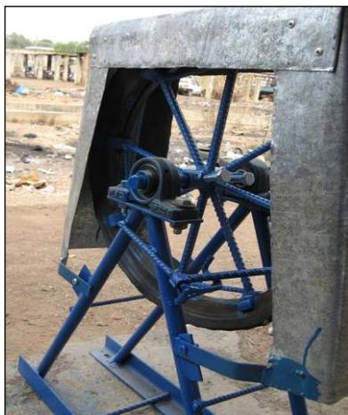
Figure 2-6 Simple metal bushings
