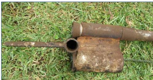
Figure 2-2 New bottom guide box, Abebe Garage Ziway
