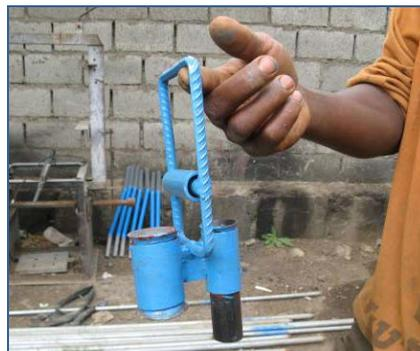
Figure 2-3 Concrete guide box (Ghana)
