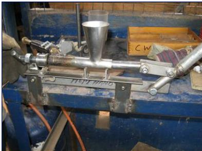
Figure 2-9 Washers produced with a small hand-operated extruder from granules or waste plastic (Ghana)
