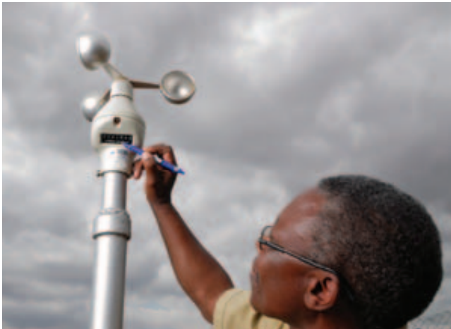
Avelini Valeriani Msoka, station manager at Same meteorological station, checks a wind speed sensor.
