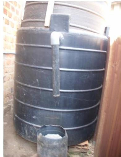
Figure 3.1. Floating drum digester in Kajansi
