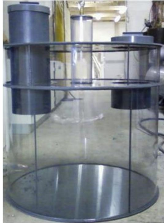
Figure 2.3. Biogas Pro digester, provided by AGAMA Energy (Austin, 2011)
