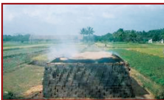
Plate E.7.25: Simple burnt clay brick clamp
