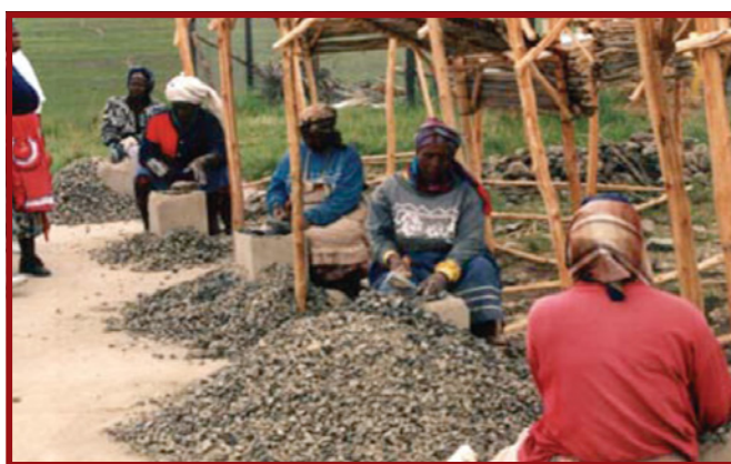
Plate E.7.37: Aggregate crushed and screened by hand
