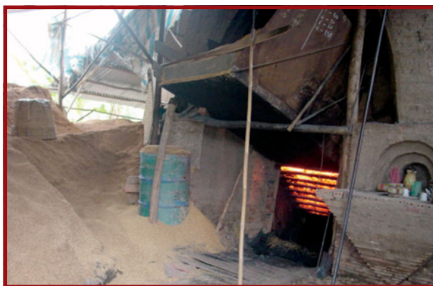
Plate E.7.24: High quality burnt clay bricks produced in small 'beehive' kilns fired by rice husk. Bricks can be fired using coal, wood or agricultural waste products
