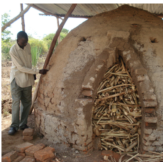
Figure 4.2: Wood arranged tightly inside a half orange kiln (Fridah Mugo)
