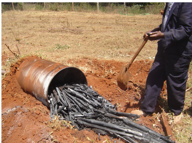
Figure 7.1: Creating charcoal from a drum kiln (Nellie Oduor, KEFRI)
