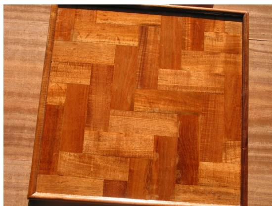
Figure 2.2: A sample of floor parquet made from Prosopis juliflora timber (Nellie Oduor, KEFRI)
