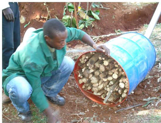
Figure 5.2: Drum kiln being tightly packed with branches of Acacia
