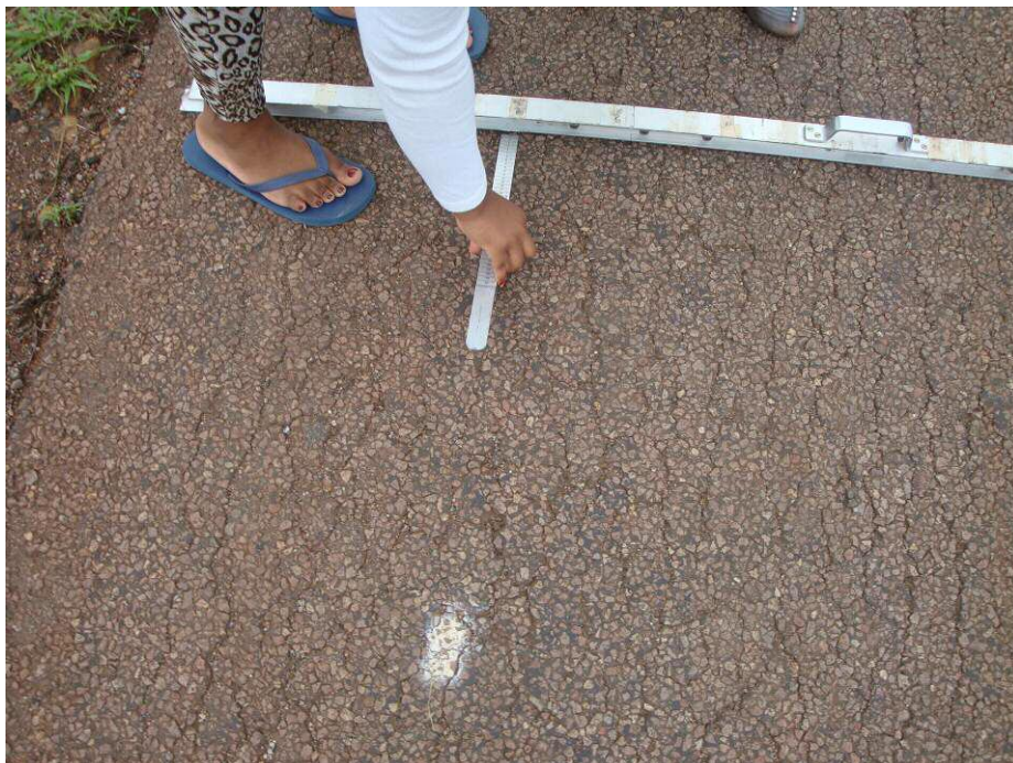
Rut depth measurement
