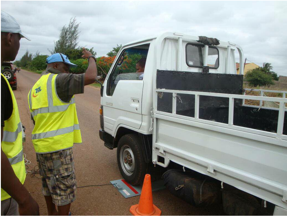
Axle load survey using portable weighbridge
