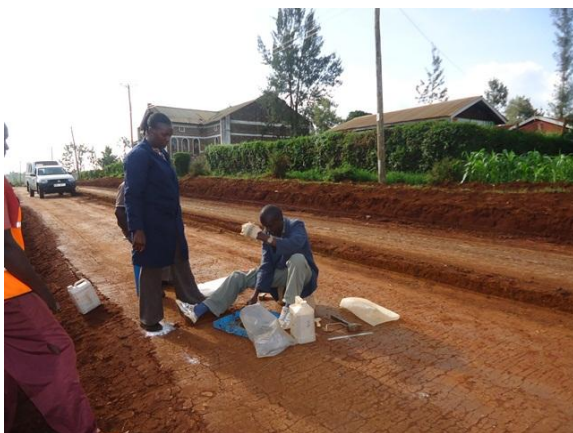
Photo 3-8: field sand displacement on the 1st layer bench
