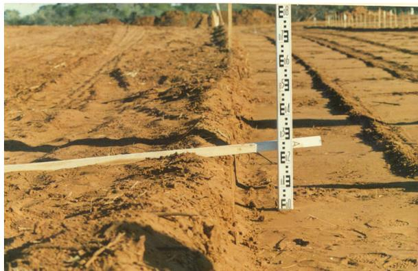
Photo 1 – A collapse settlement in excess of 150 mm was obtained along a section of the Serowe-Orapa road after compaction to near refusal by a 25 kJ high energy impact compactor.
