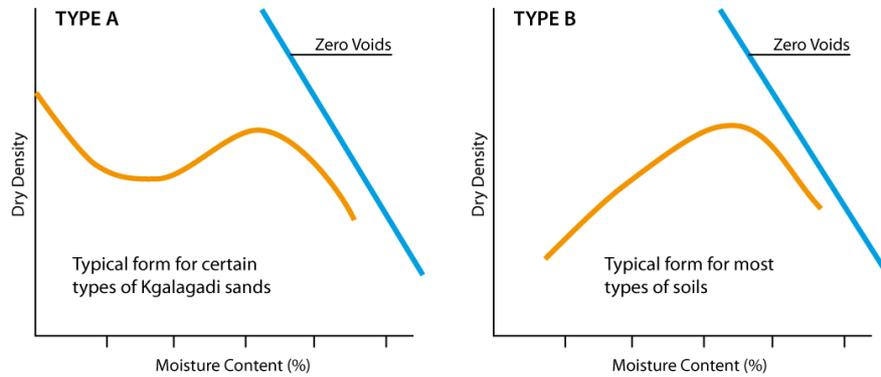
**Figure 3-10: Typical forms of compaction curve for sands.**
