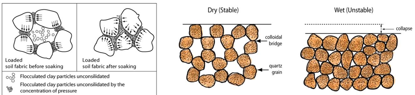
**Figure3-9: Graphical illustration of collapsible sand fabric (Brink, 1985) and mechanism of collapse**
