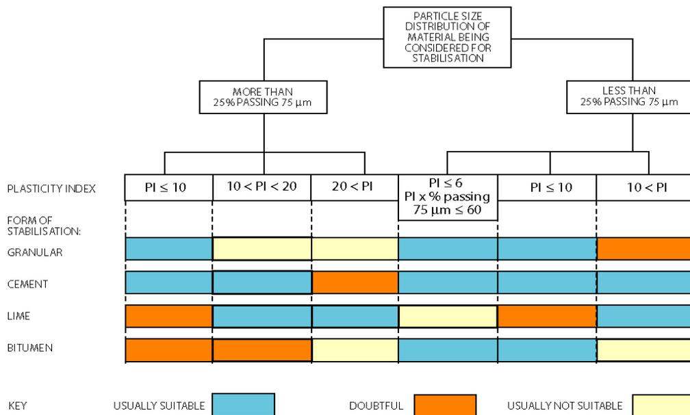
**Figure 5-2: Guide to the method of stabilization (Austroads, 1998)**
