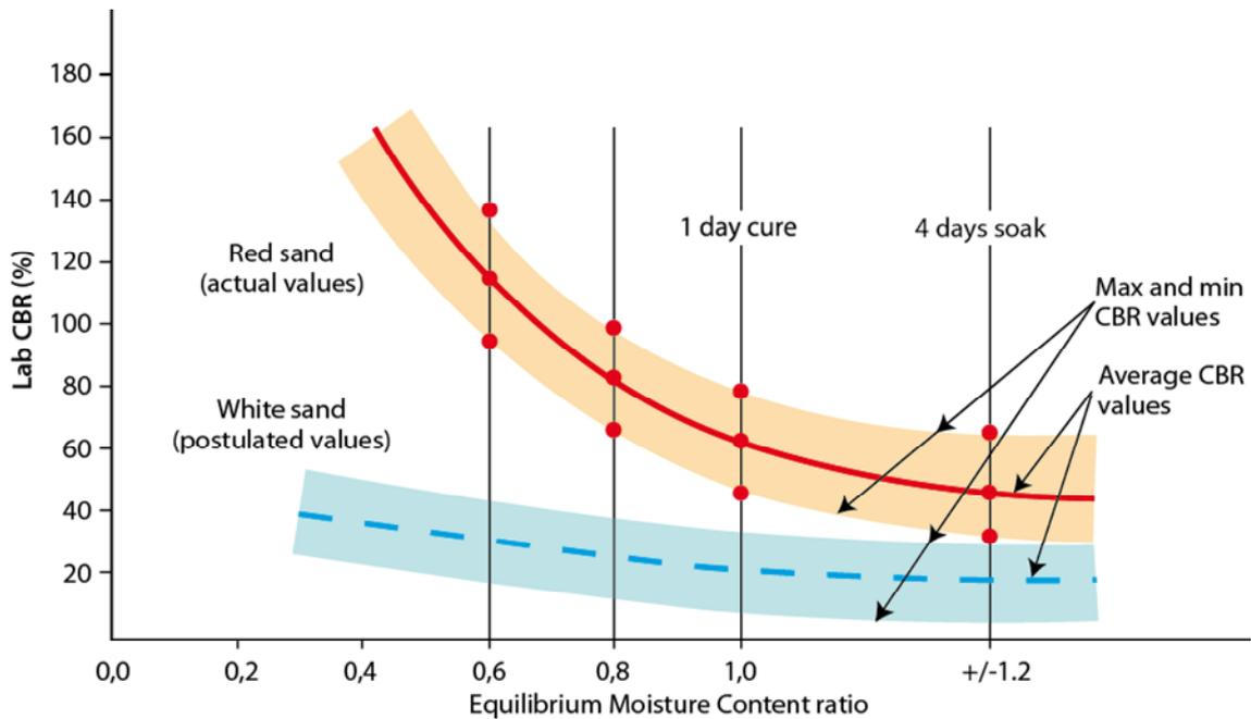
**Figure 5-1: CBR of Kalahari sand sample at various moisture content ratios**
