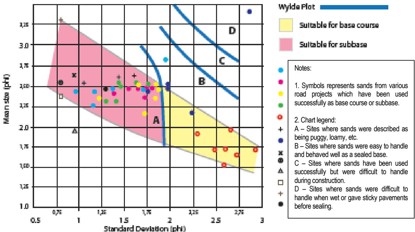
Figure 6-1: Classification of sands based on grading (Metcalf and Wylde, 1984)
