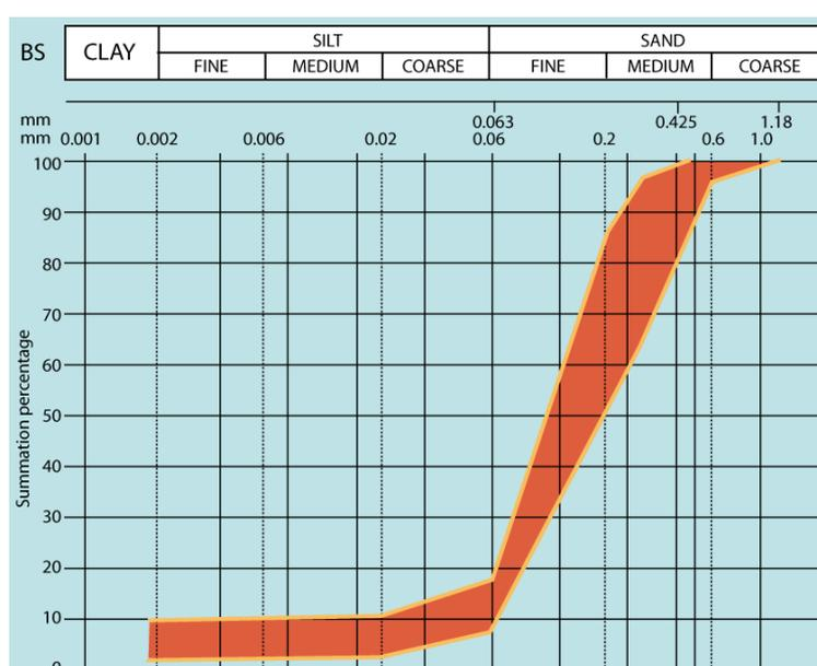
**Figure 3.7 – Grading envelope for typical Kalahari sand types found in Botswana**
