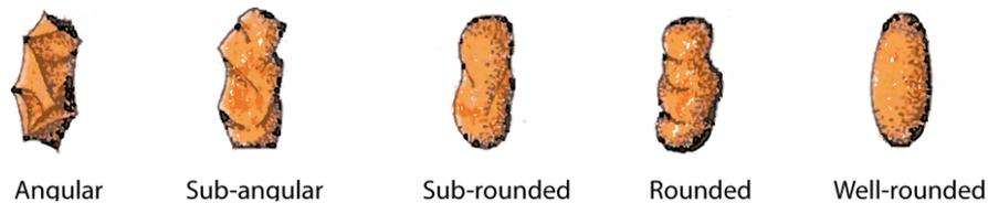
**Figure 3.4 – Degree of particle roundness**
