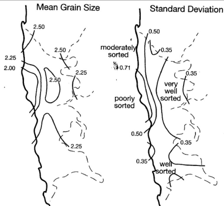
**Figure 2-6: Grain size and sorting of Namib Sand Sea sands (Lancaster, 1986)**
