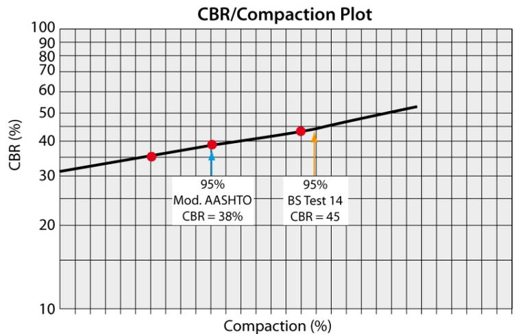
Figure 4-2: CBR/compaction relationship
