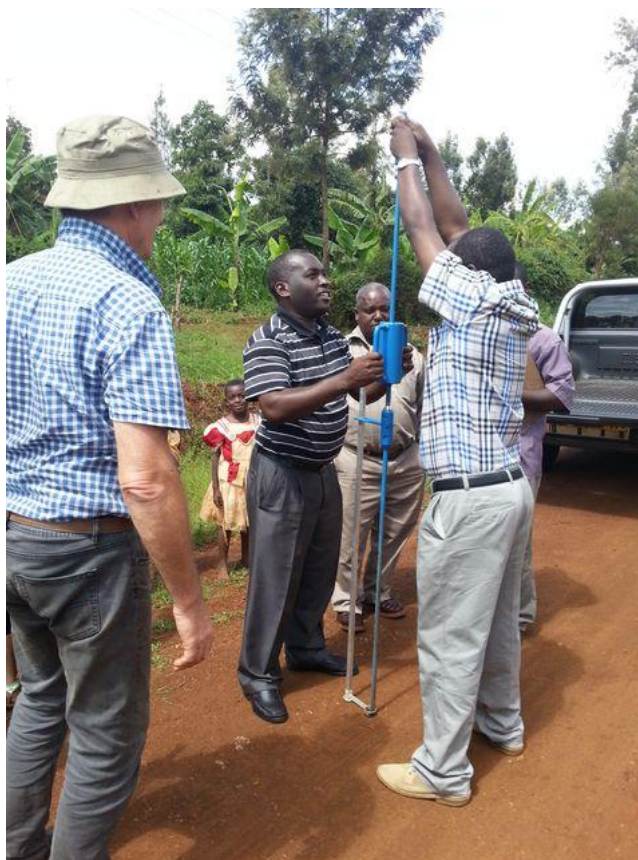
Picture 1: Regional Managers doing DCP test
