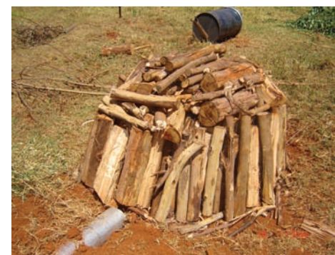
Left: Wood arranged upright for Casamance kiln (Nellie M. Oduor, KEFRI)
