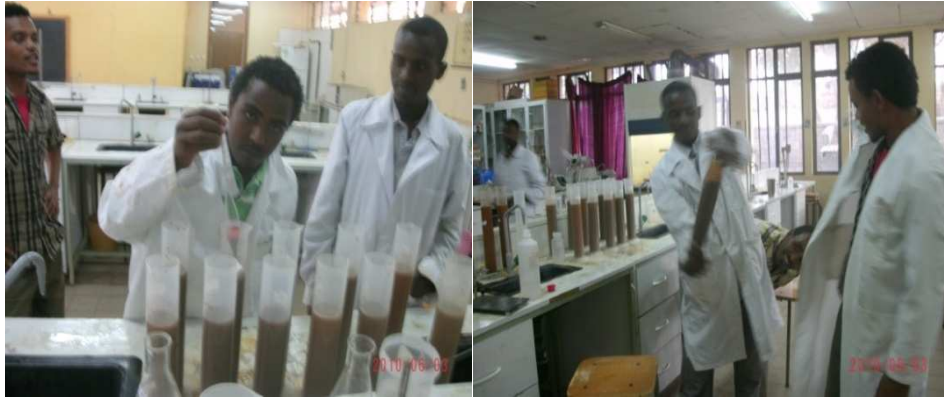
Figure 10 Sediment grain size analysis using Hydrometer
