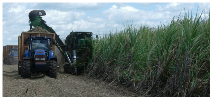
Figure 1: Harvester Collecting Sugarcane and Filling the Tractor Trailer Source: Pedro Ninô de Carvalho
