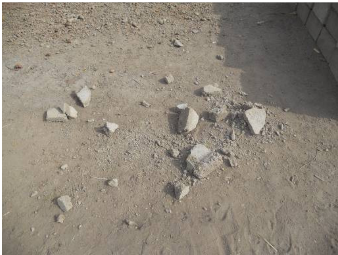
Plate 3 The result of inadequate curing; very poor quality blocks
