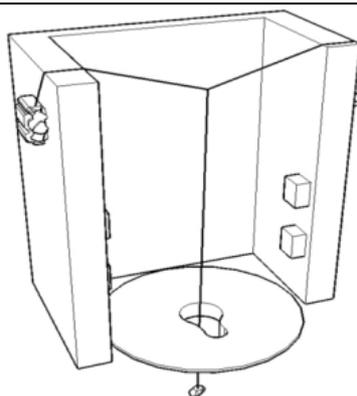
**Figure 19: Latrine design with protruding bricks for support, and string for blind user to locate drop-hole**
