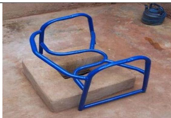
**Figure 20: Moveable toilet seat made of gi pipe**
