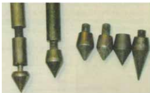
Photo 2A-1: Typical cones and problems
