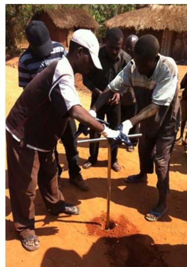
Handling of auger
