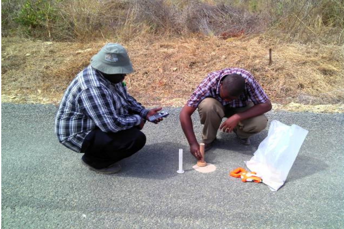
Figure 5: Sand Patch Testing
