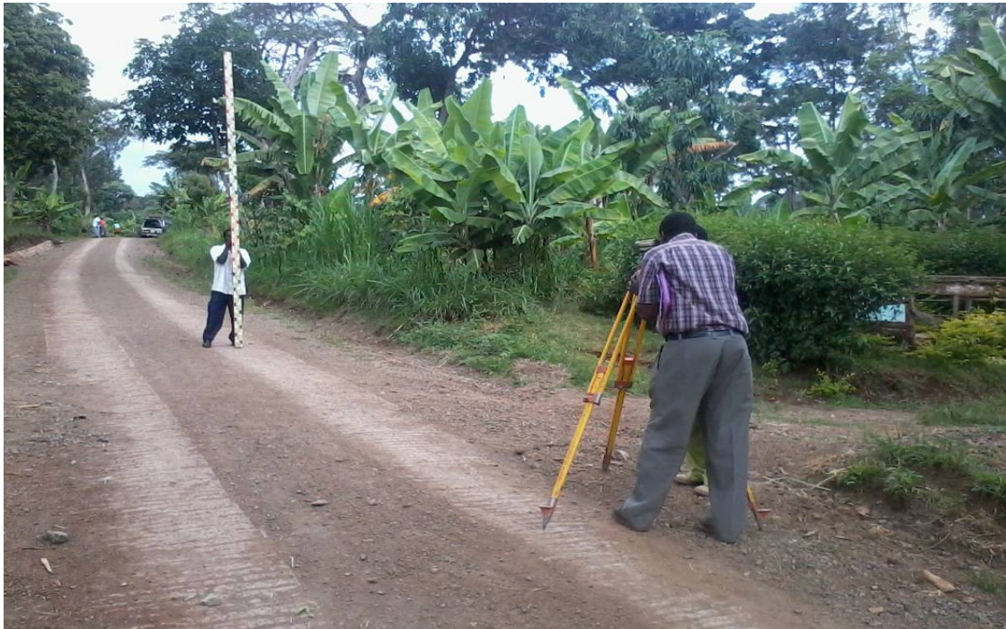
Figure 2: Surface Profile Measurement
