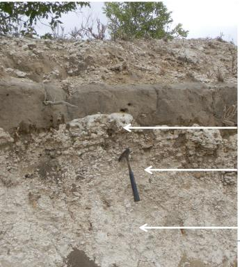
There are various types of calcrete used in LVR construction as sub-base, base and w/c gravel
