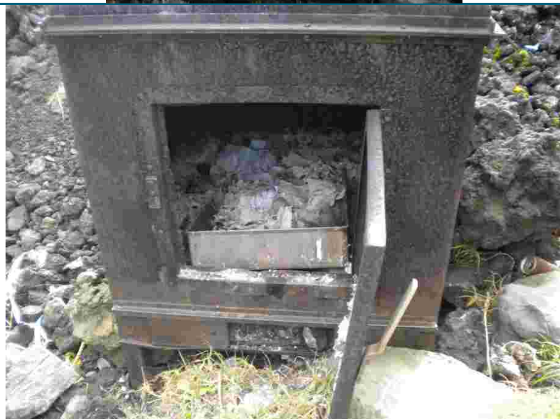
Figure 8 – Residues of incineration of health care waste.
