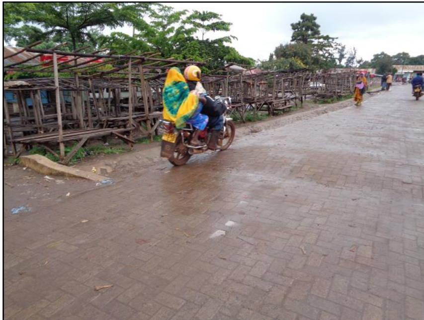
Photo 12: Boda-Boda Passing around the End of a Speed Hump on Paving Bricks (L-K)
