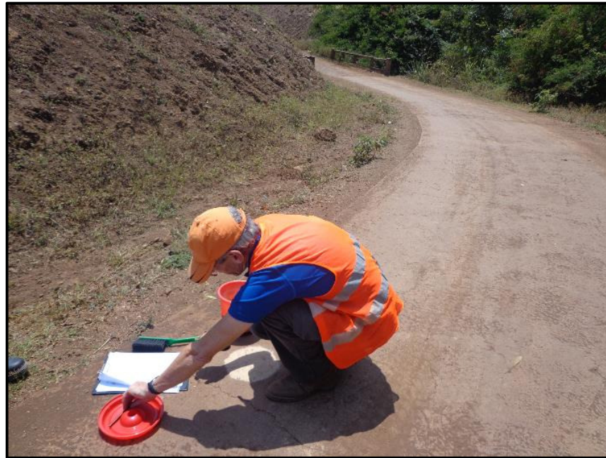
Photo 3: The 'Sand Patch Test' (Lawate-Kibong'oto)
