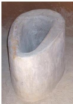
**Cement bowl made with mould**
