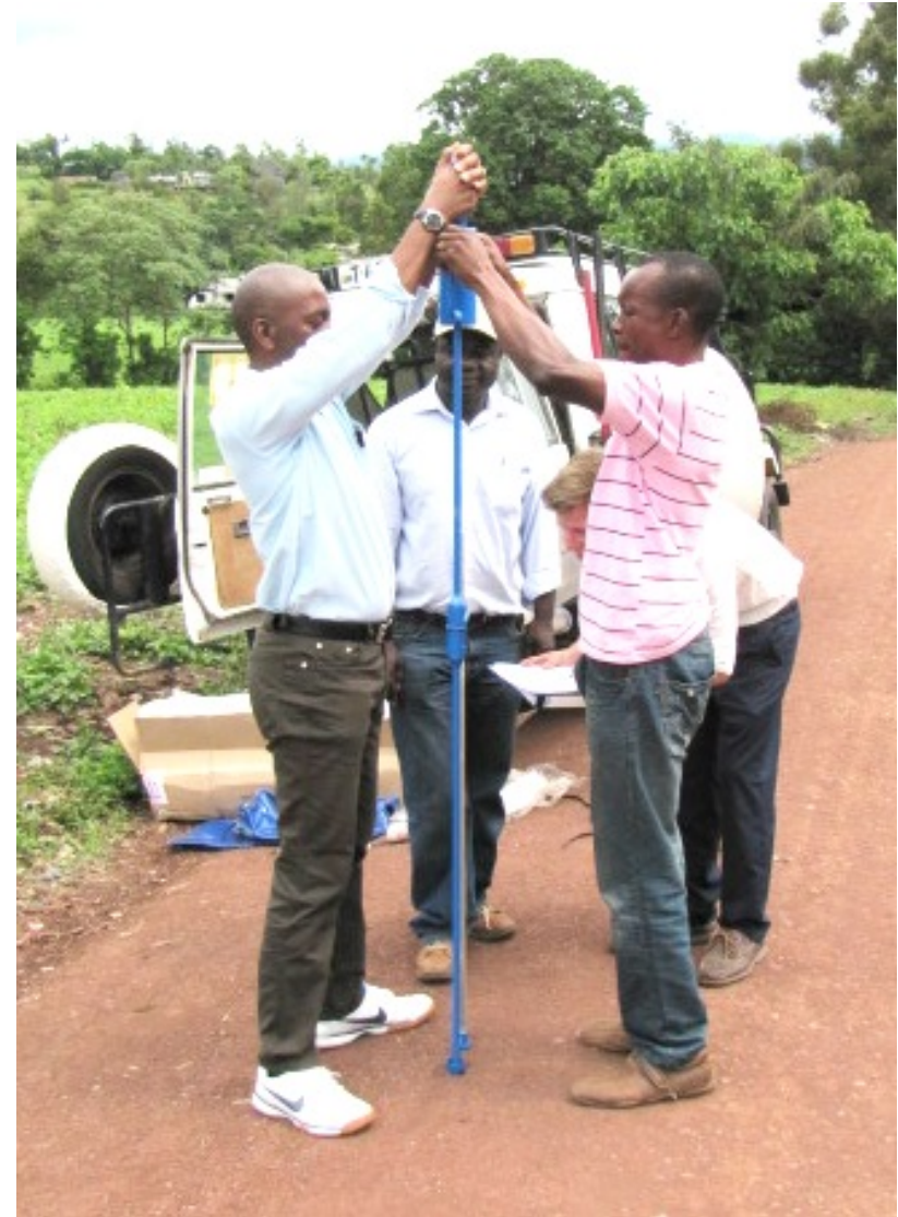
DCP test in process
