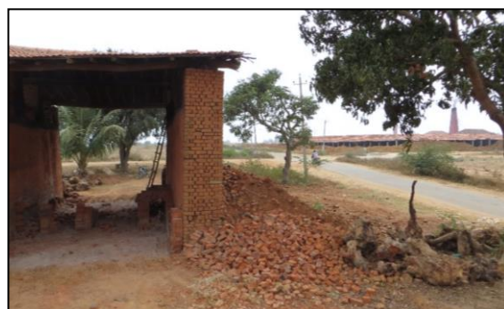
Fig.1 - Kiln heterogeneity in Karnataka: open kiln (foreground) and Hoffman kiln (background)
