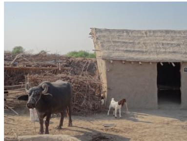
**Acceptability** – This shelter was weatherproof but with only one opening for the doorway, light and ventilation was limited inside the shelter. No door was provided in the doorway so security was an issue. This shelter was not part of an integrated programme, so space for cooking and WATSAN were not considered.
