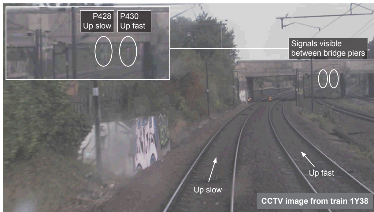
Figure 8: First sighting of signal P428 (courtesy VTEC)
