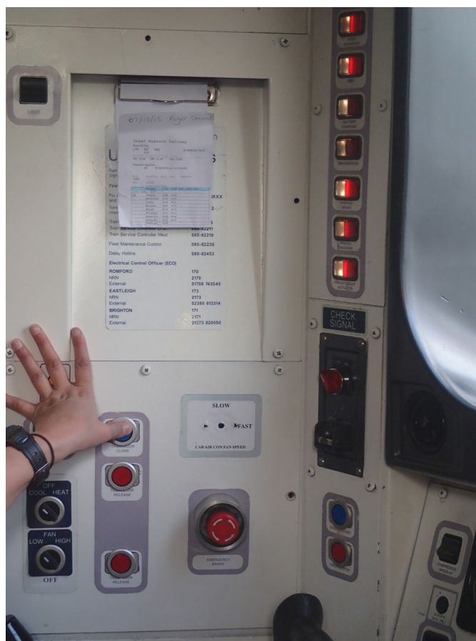
Figure 25: Train driver pressing the button to initiate the door closure
