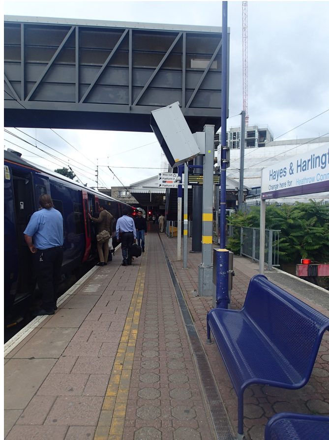
Figure 27: Image showing a train driver checking the platform during the dispatch process. Various methods of DOO dispatch were observed by RAIB (door open / door closed with window open and closed).
