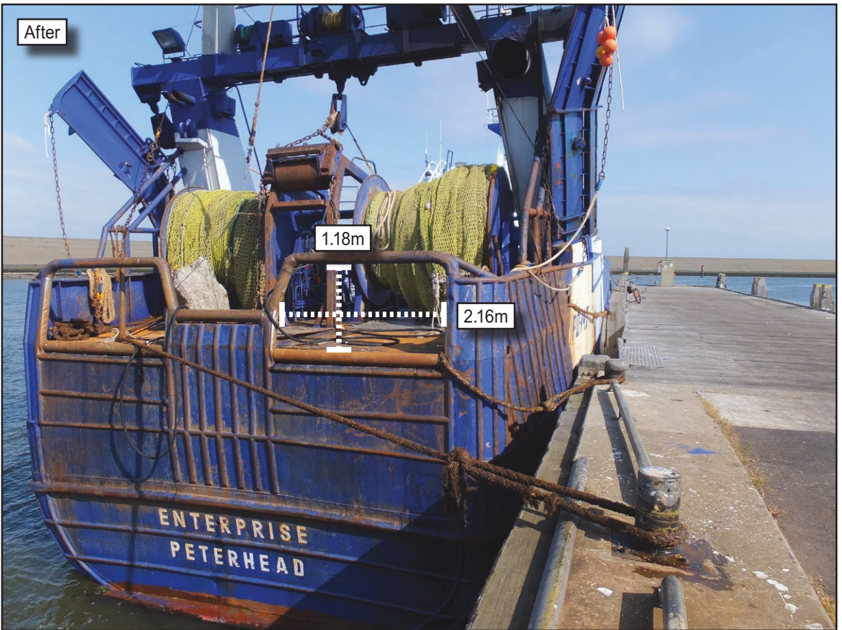
Figure 4: Enterprise before and after conversion to a stern trawler
