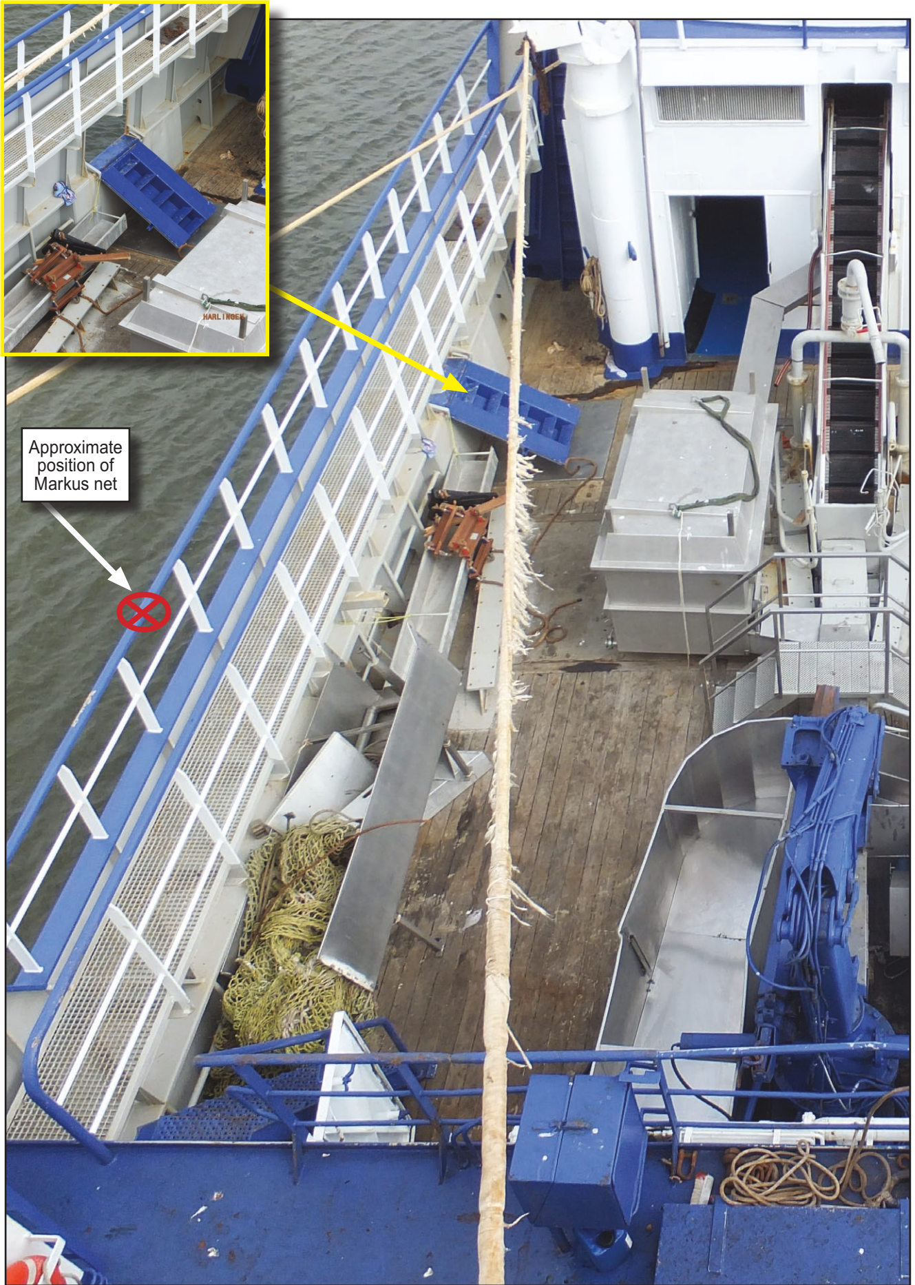
Figure 3: Pilot ladder and Markus net deployment positions (inset: opening for pilot ladder)
