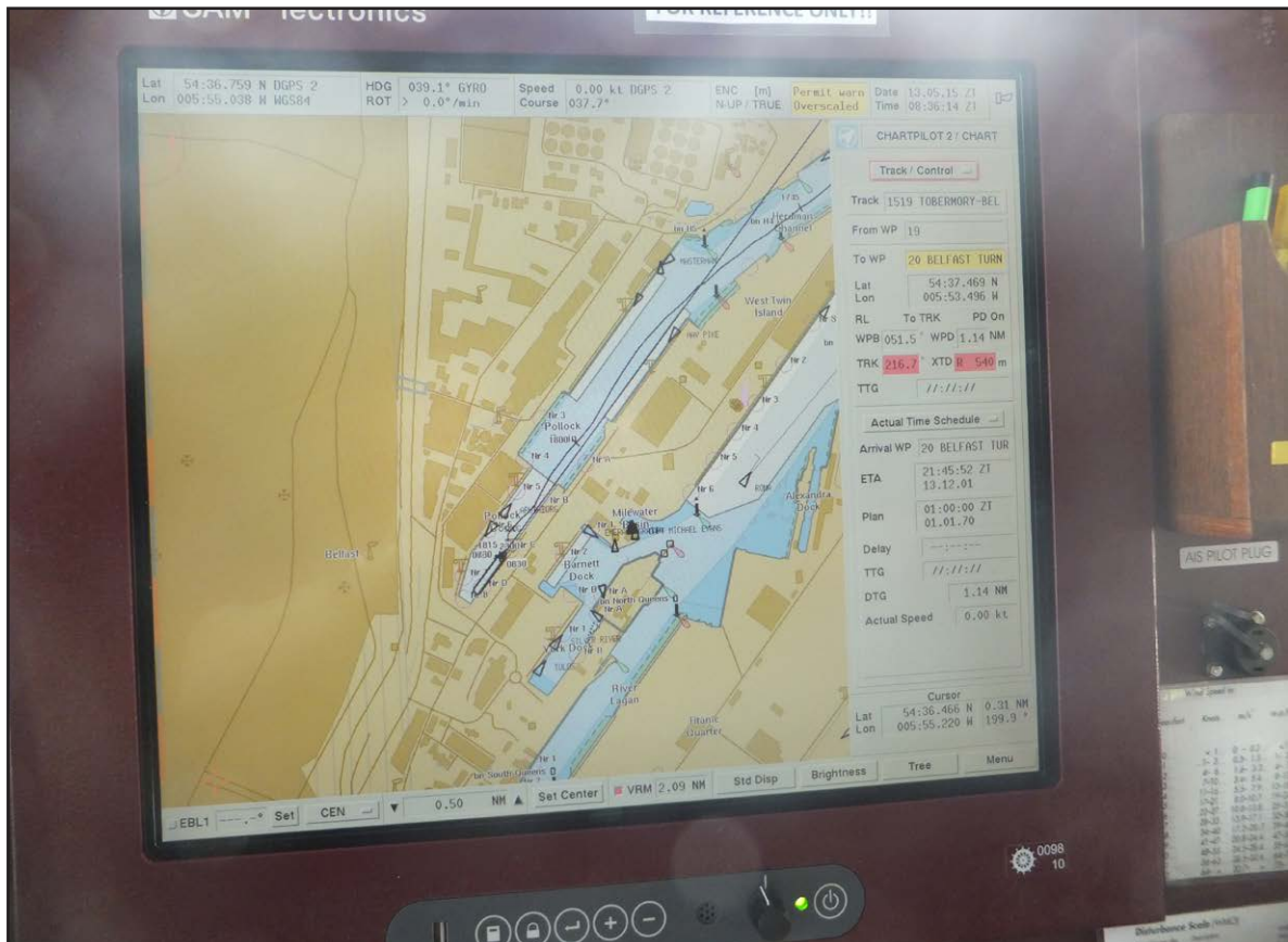
Figure 12: Hamburg's ECDIS display showing AIS information
