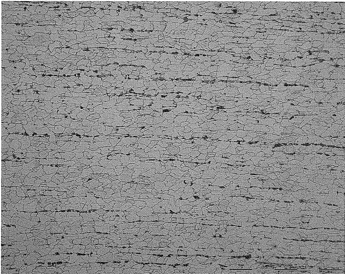
PHOTO 4 - FERRITE/PEARLITE STRUCTURE X100 MAGNIFICATION
