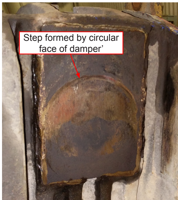
Figure 11: Worn axle box longitudinal wear plate
