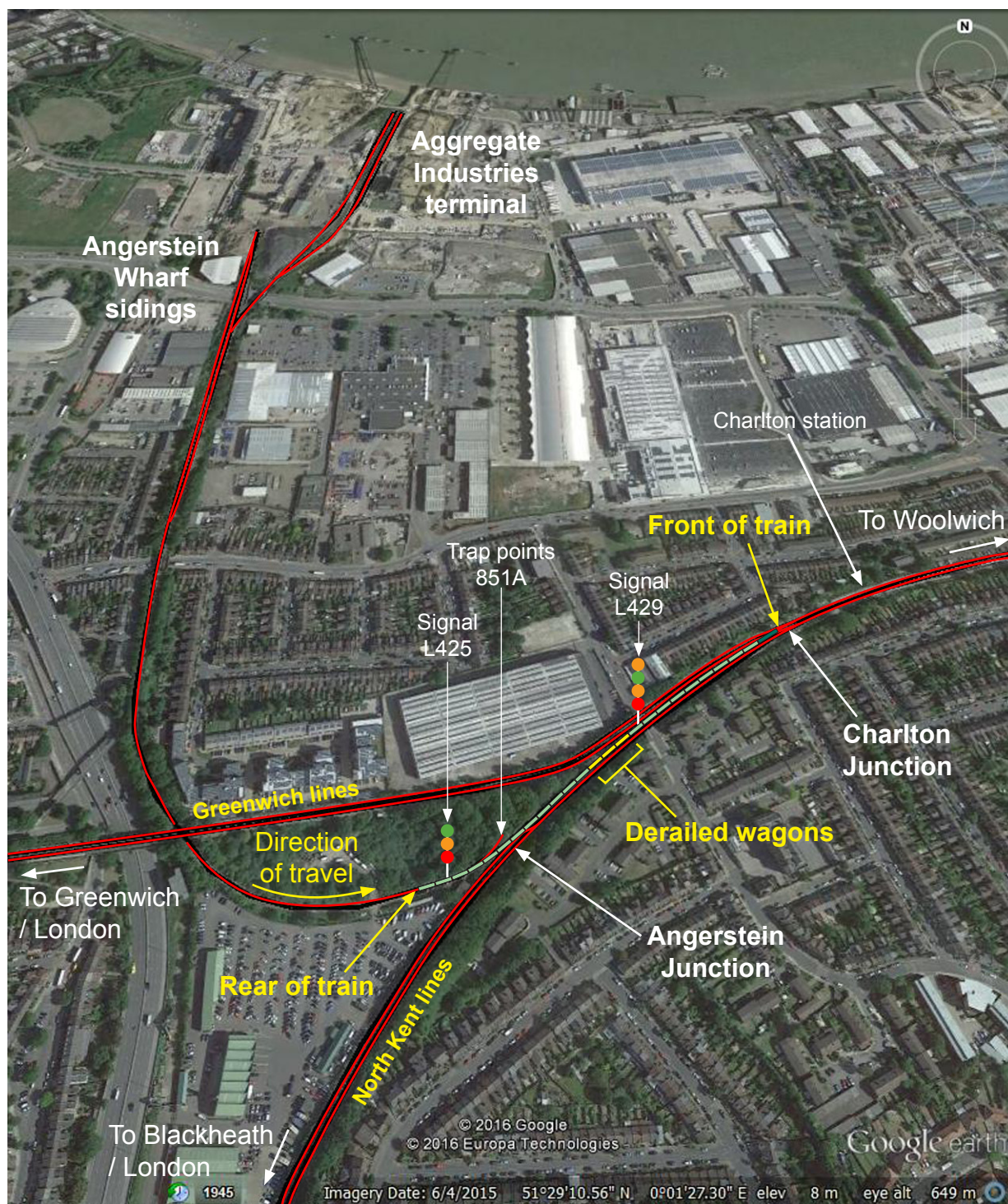
Figure 3: Google Earth image showing track layout and selected signals (showing train location after stopping)
