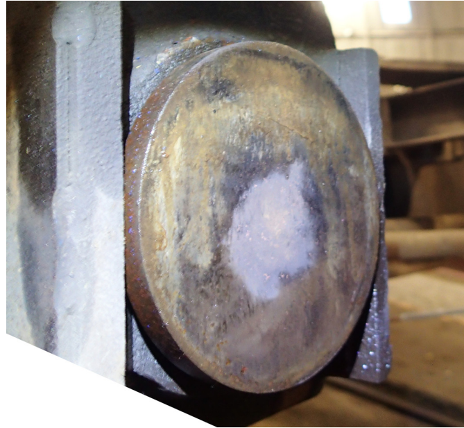
Figure 12: Damper wear face
