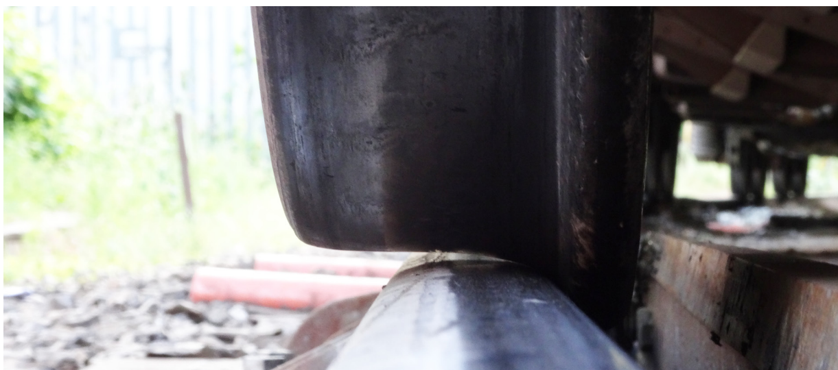
Figure 16: Wheel with working suspension starting to flange climb at the point of derailment
