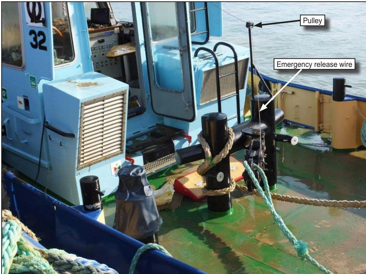
Figure 9: Towing hook emergency release wire
