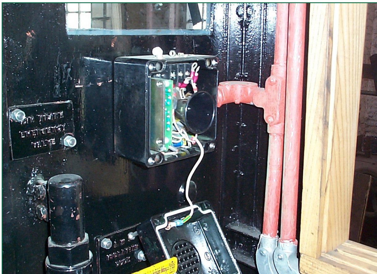
Figure 15: The AWS audible warning indicator unit fitted to Tangmere during its restoration (photograph courtesy of Resco Railways)
