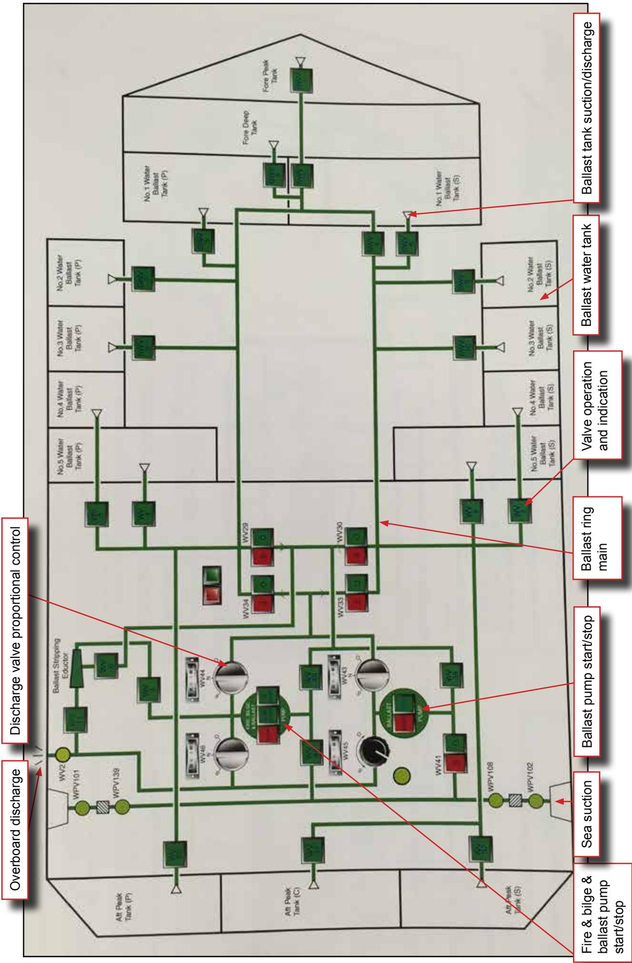
Figure 23: Ballast system diagram
