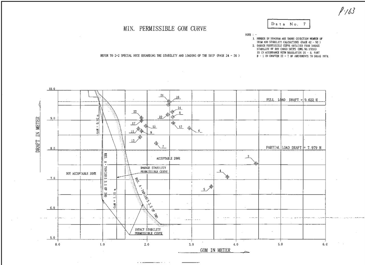
**Figure 25:** Minimum permissible GM curve
