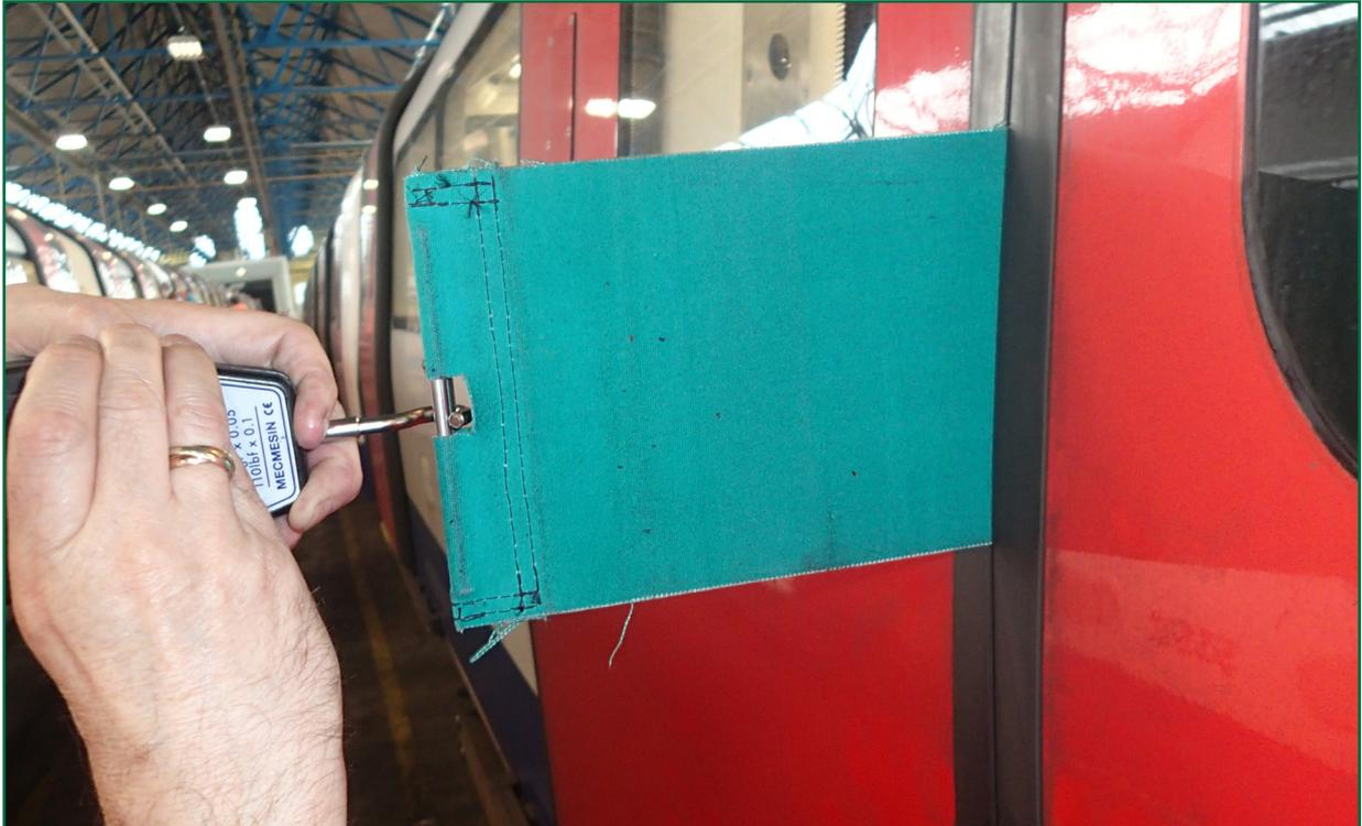
Figure 14: Pull-out testing with canvas piece
