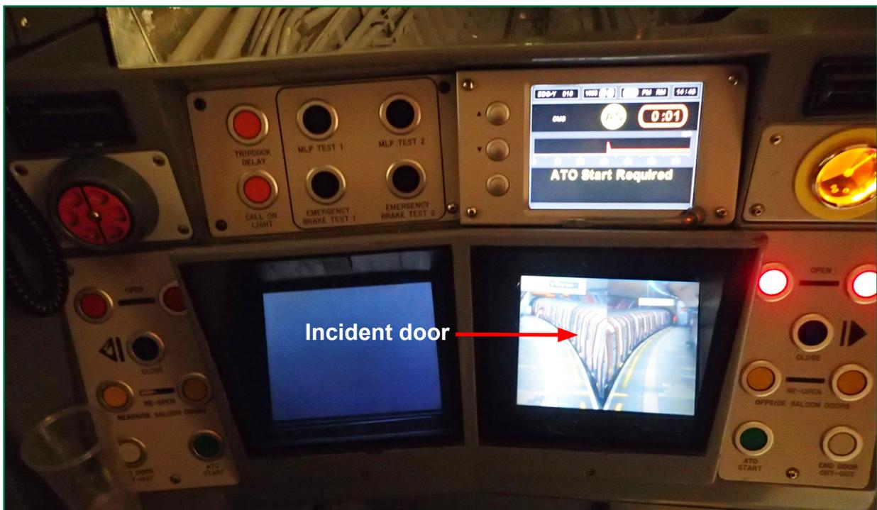
Figure 16: Train operator cab display at Clapham South station (image does not show accident situation)
