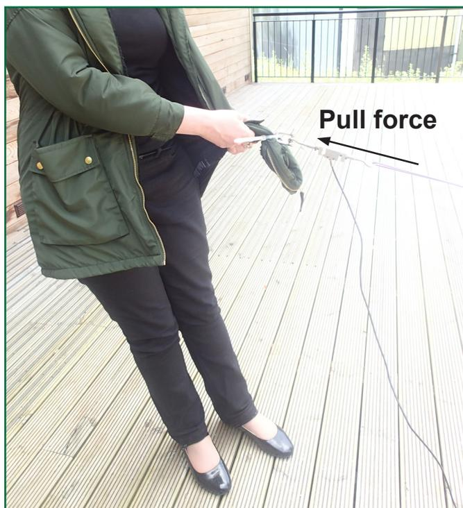
Figure 12: Testing pull-out force applied by person wearing incident coat
