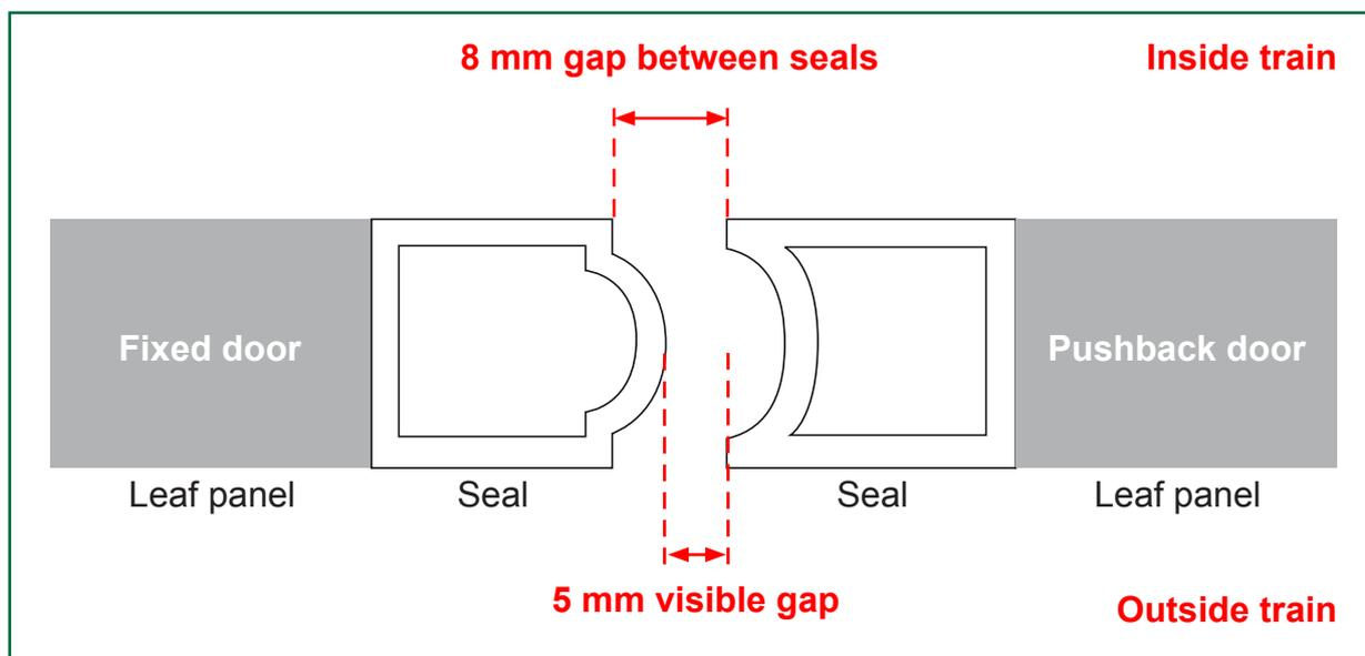
Figure 15: Door seal gap for loss of interlock
