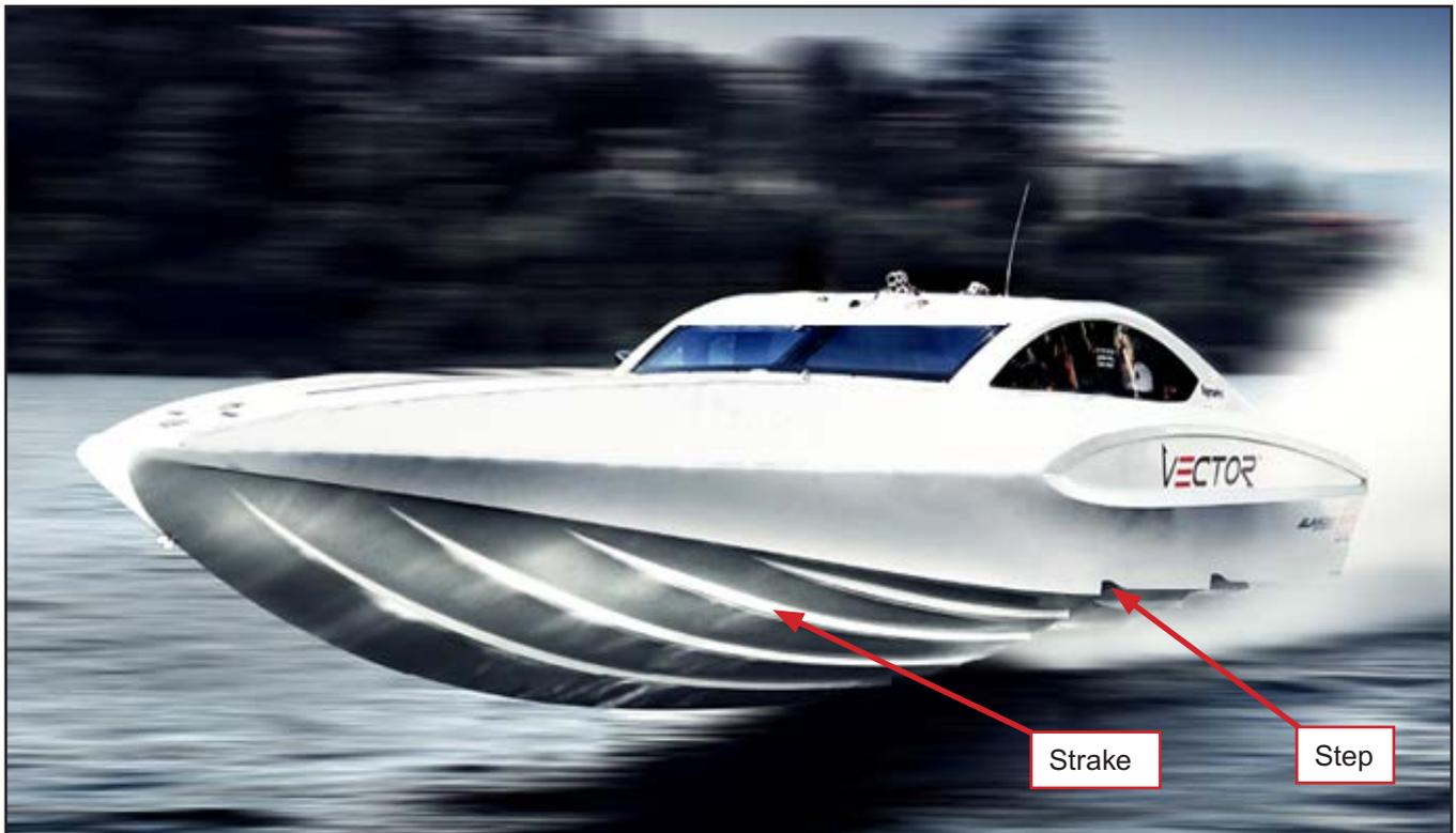
**Figure 1:** Stepped hull with multiple strakes
