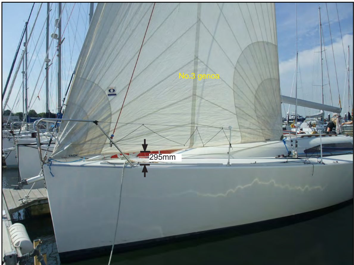
Figure 11: Gap between the foot of No.3 genoa and the deck
