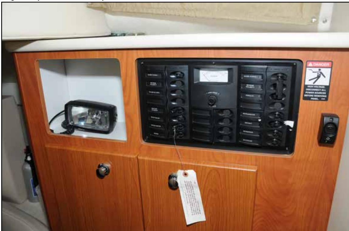
Figure 12: Electrical distribution panel
