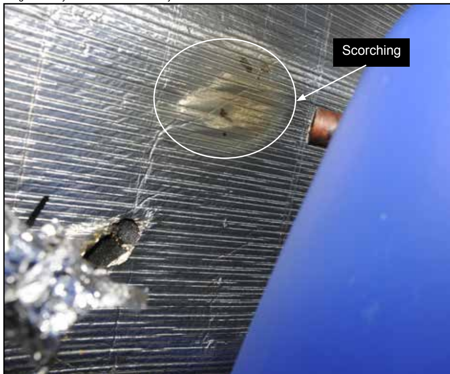
Figure 16: "Scorch" marks engine bay on bulkhead
