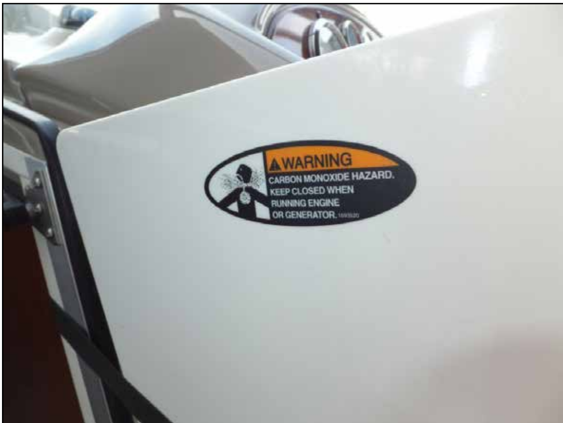
Figure 20: Warning of CO hazard on accommodation door
