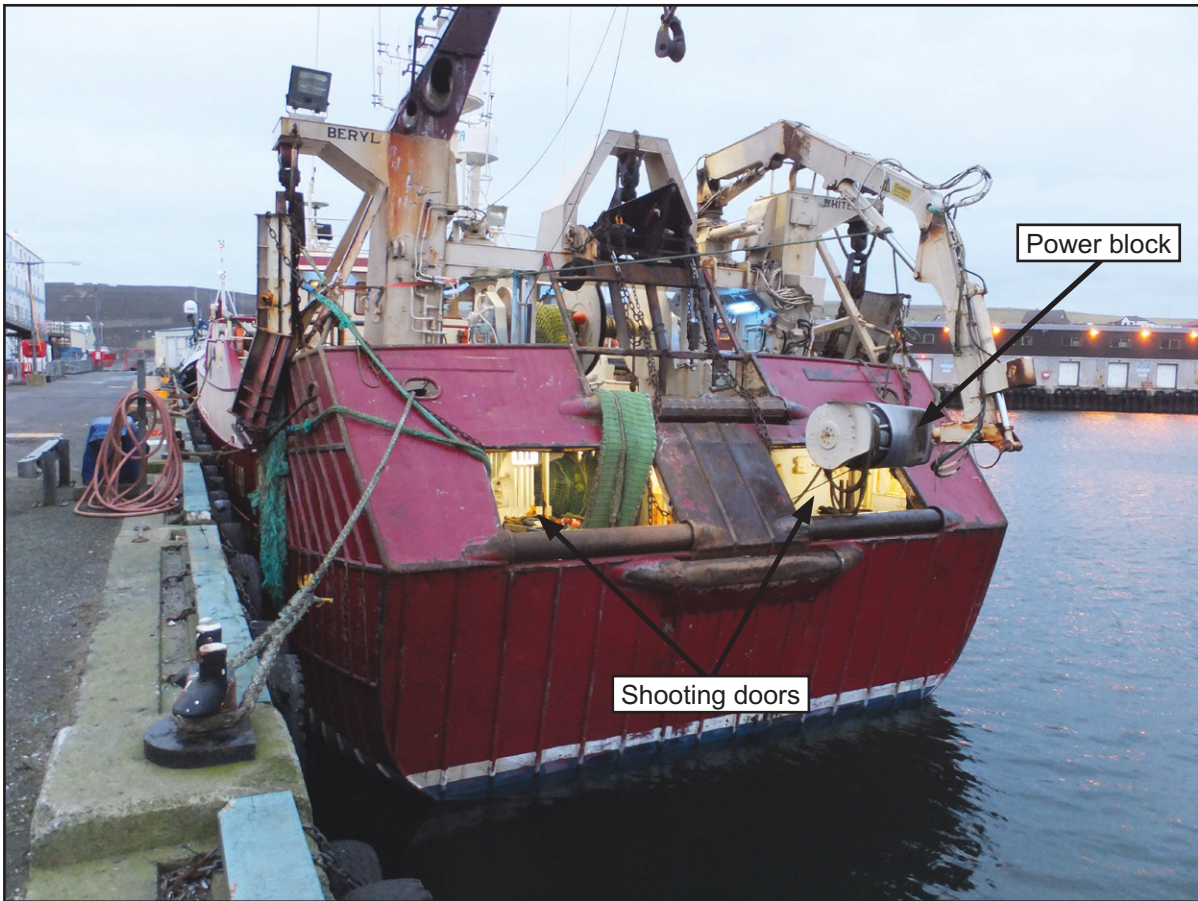
Figure 4: Beryl's stern showing the shooting doors and power block
