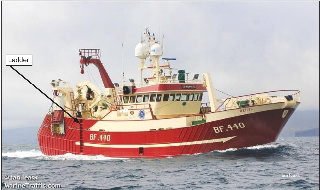
Figure 10: Vertical ladder built into Beryl's side plating (note - an identical ladder was sited on the vessel's port side)
