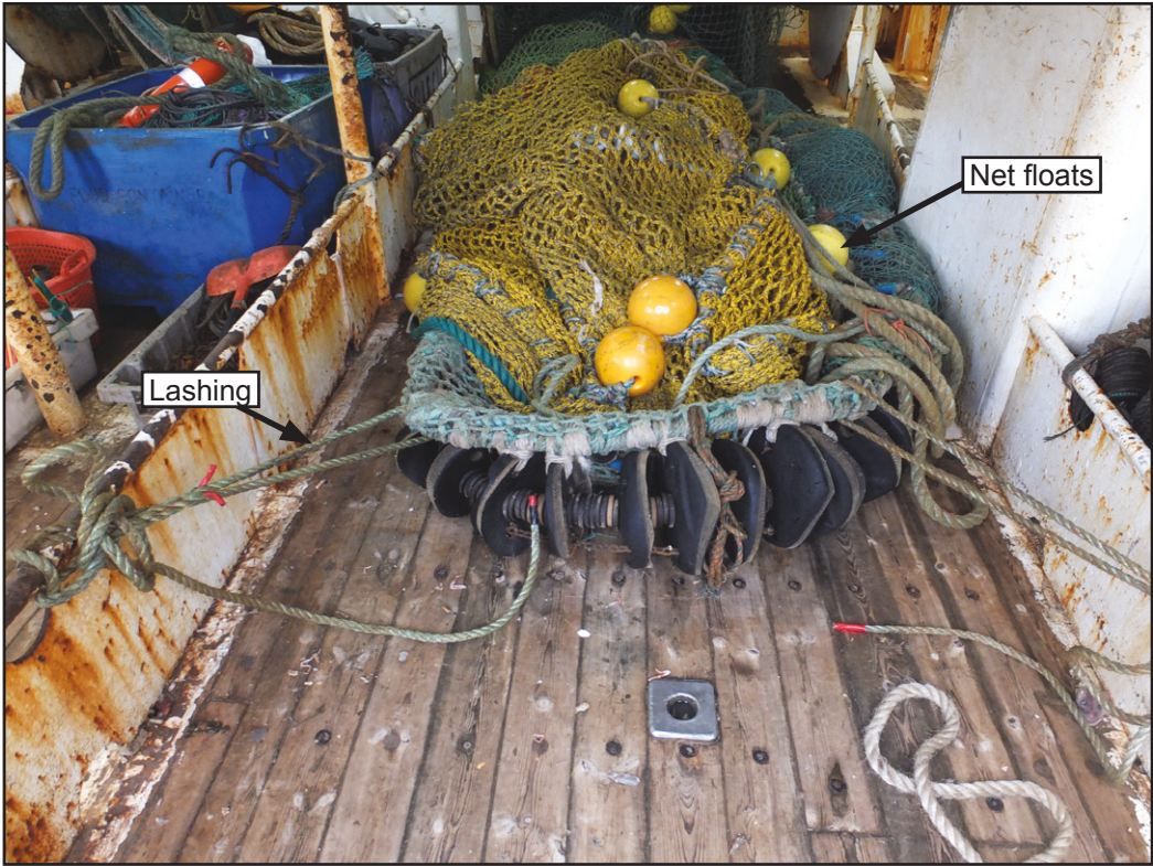
Figure 2: Starboard trawl ground gear lashed into the track
