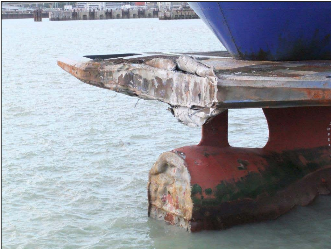
Figure 6: Damage to bulbous bow and “cow-catcher”
