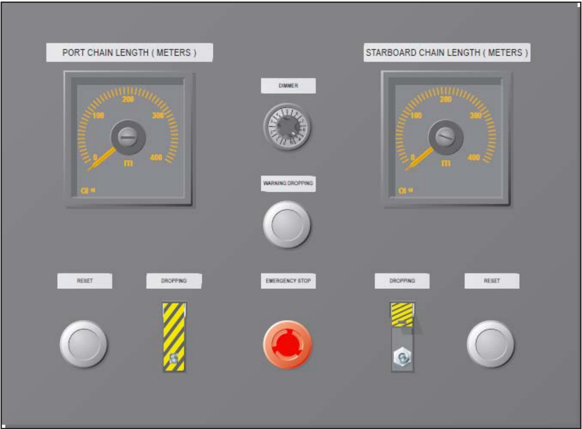
Figure 5: Bridge remote anchor release controls
