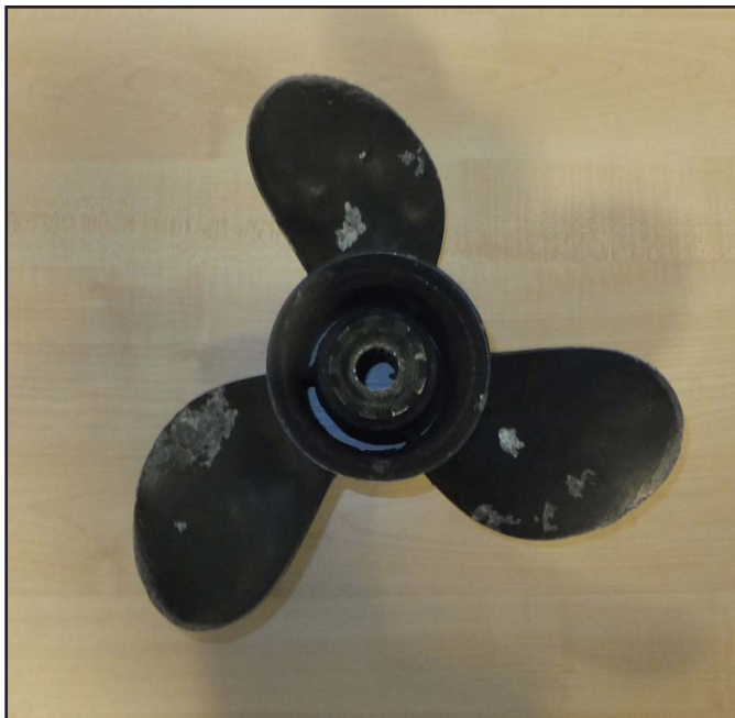
Figure 6: Three-bladed aluminium alloy propeller
