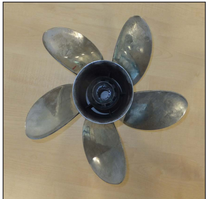
Figure 7: 'HighFive' five-bladed stainless steel propeller
