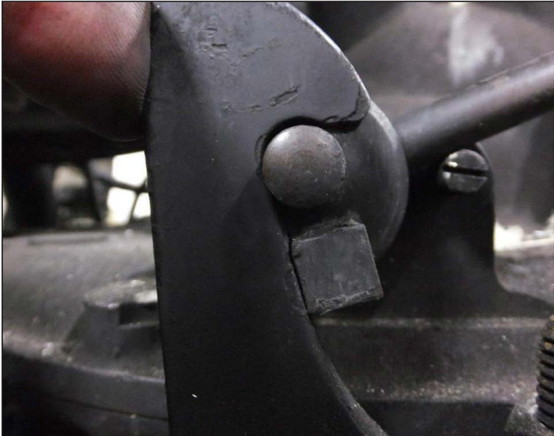
**Figure 3b:** Photograph showing burner unit latching mechanism (closed)
