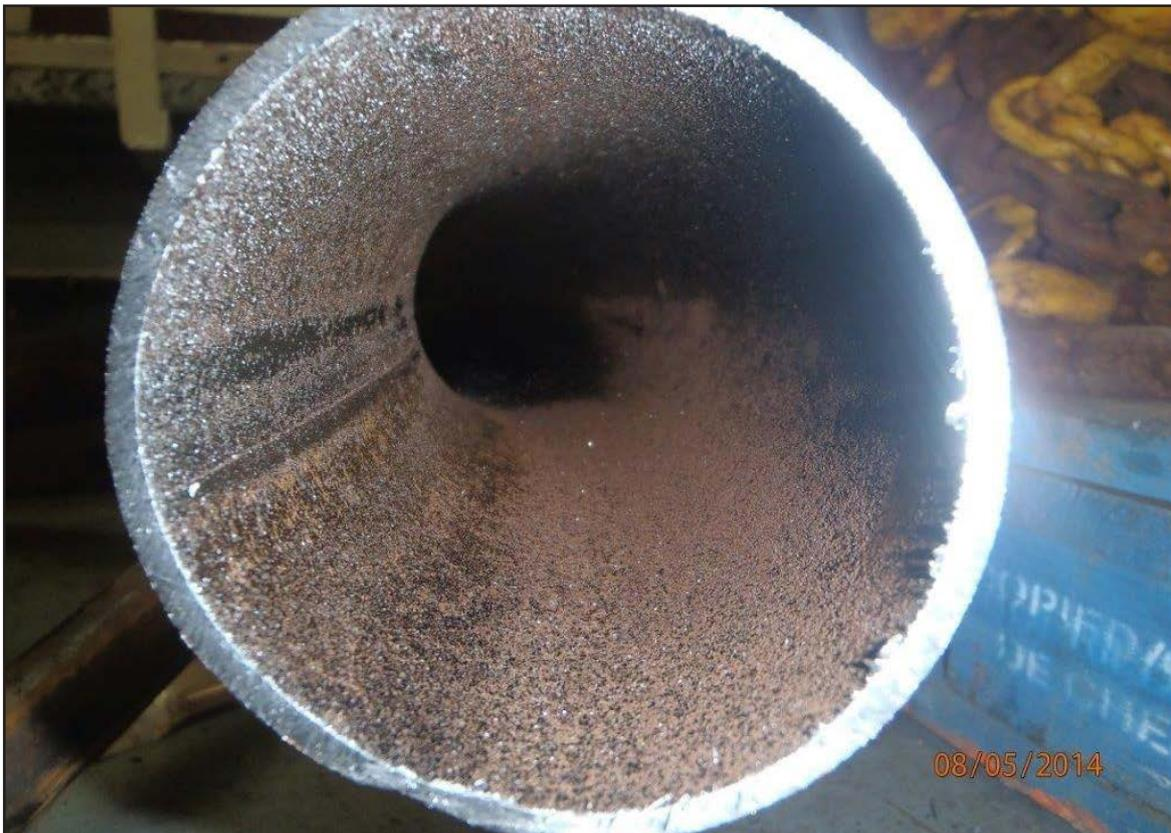
**Figure 11:** Photograph of internal surface of damaged section of port thermal oil heater coil
