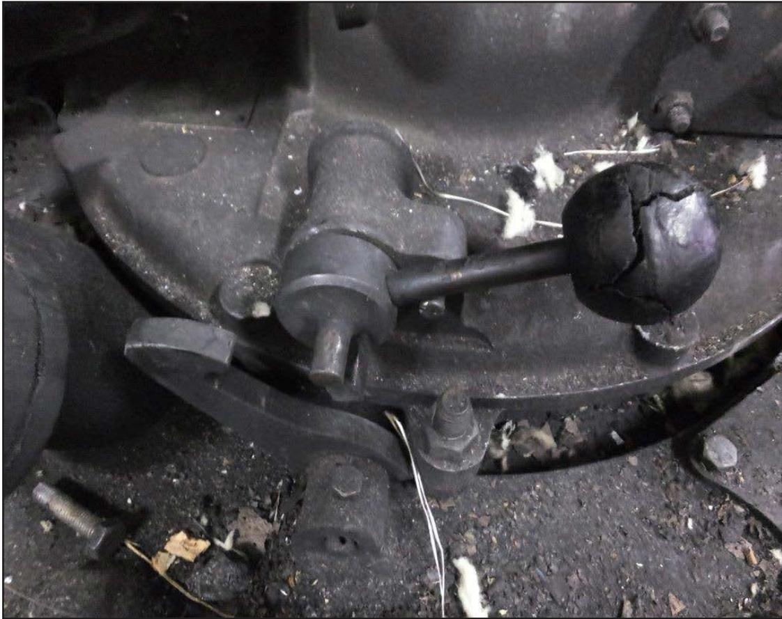
**Figure 3a:** Photograph showing burner unit latching mechanism (open)
