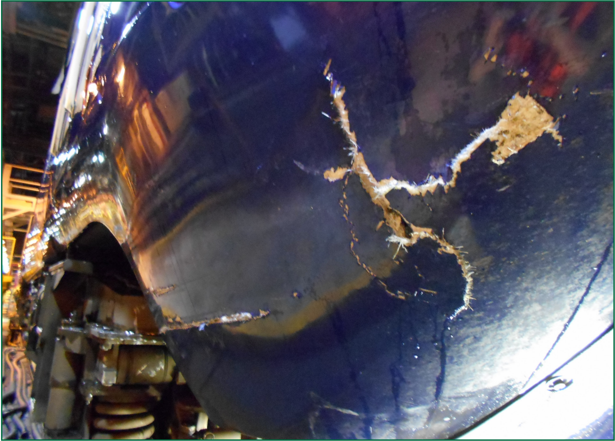
Figure 4: Damage to power car 43160 (courtesy of First Greater Western)
